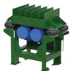
The empty box, carton or drum is rolled into position over the grid top which is in the lowered position. Upon starting, the grid deck is raised by inflating air mounts and the load is elevated off the roller conveyor surface. The contents are then compacted or settled inside the container. Upon completion of the vibrating cycle, the container is lowered back onto the conveyor and advanced to the next operation.
